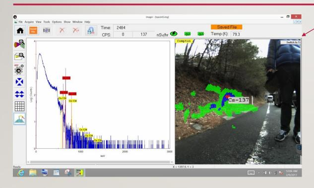
GeGI detected backward contamination at Point 4 so measure backward
